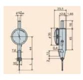
Model L (mm) PC-1AV 21.4 PC-1BV 22.4 PC-1LV 43.0 PC-2V 12.0
